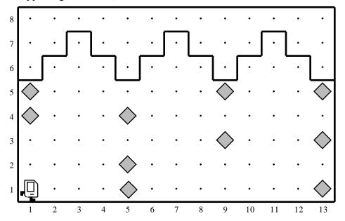
When Karel is done, the missing stones in the columns should be replaced by beepers, so that the final picture resulting from the world shown above would look like this:
